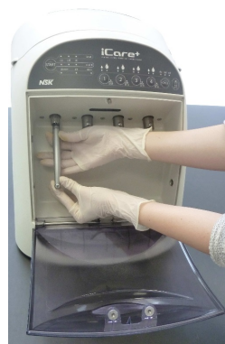
Fig.15 – Screwing the retaining nut
